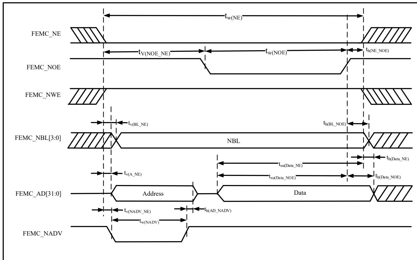
Table 4-54 Asynchronous Bus-Multiplexed PSRAM/NOR Read Operation Timing<sup>(1)(2)</sup>
