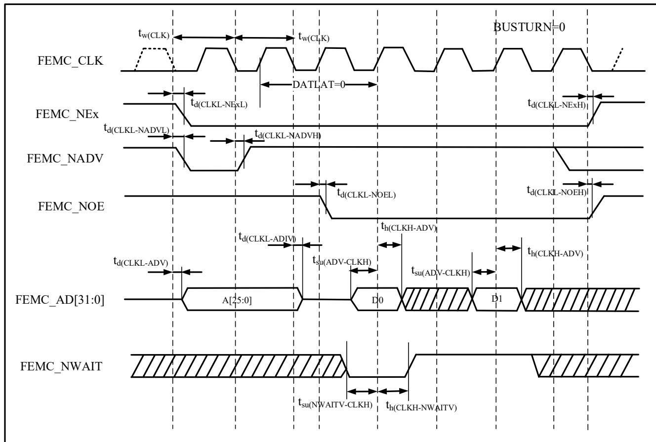
Table 4-58 Synchronous Bus-Multiplexed NOR/PSRAM Read Timing<sup>(1)(2)</sup>
