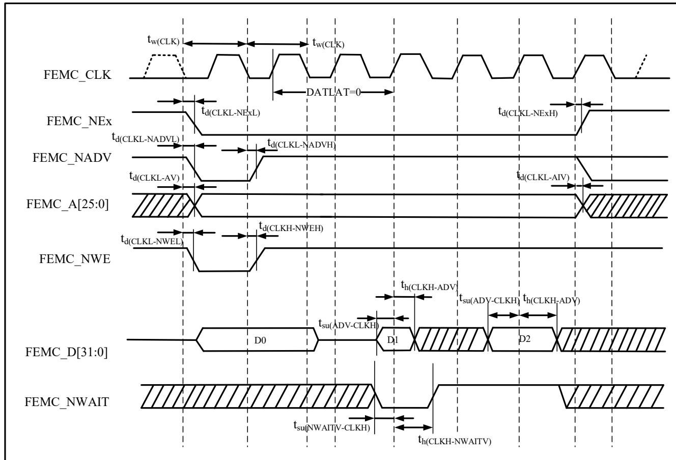
Table 4-57 Synchronous Non-Multiplexed PSRAM Write Timing<sup>(1)(2)</sup>
