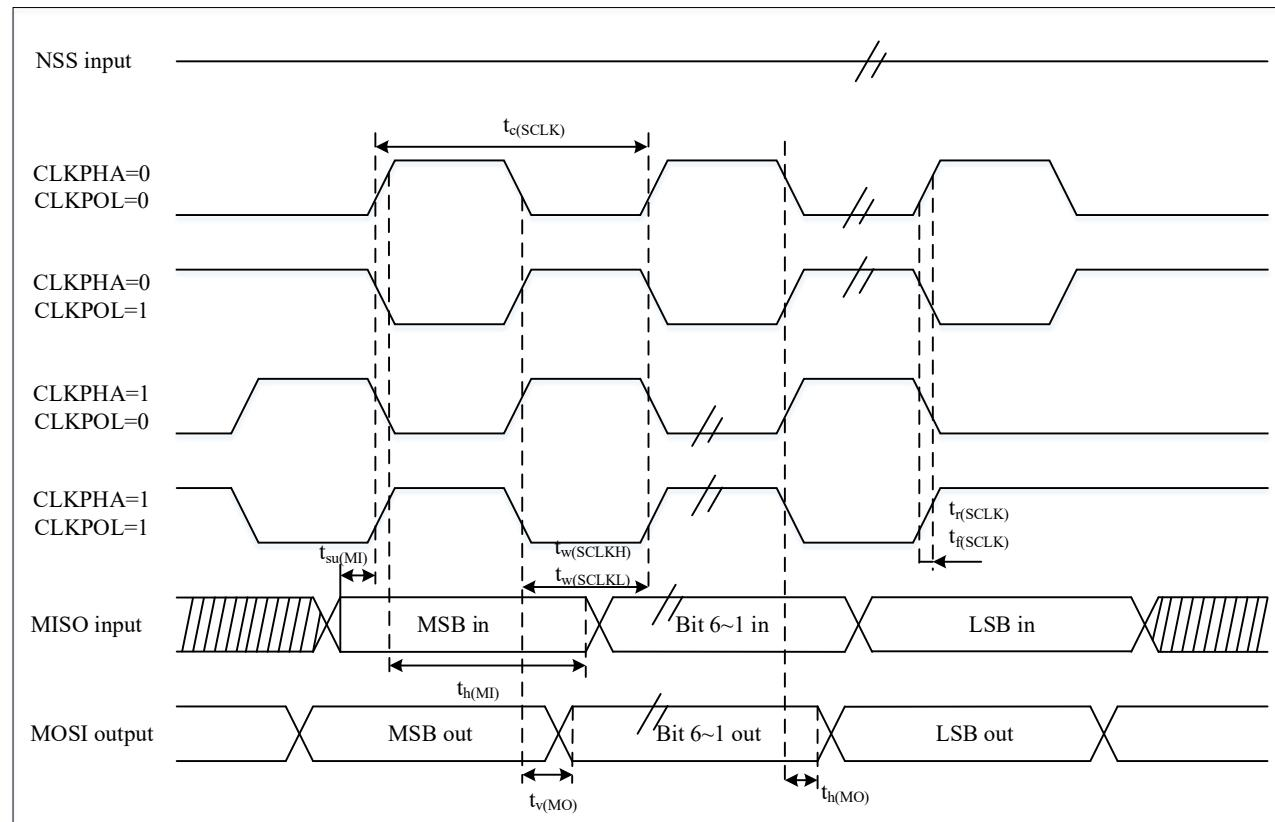
Note: Measurement points are set at 0.5VDD, with external load capacitance (CL) of 30pF.
