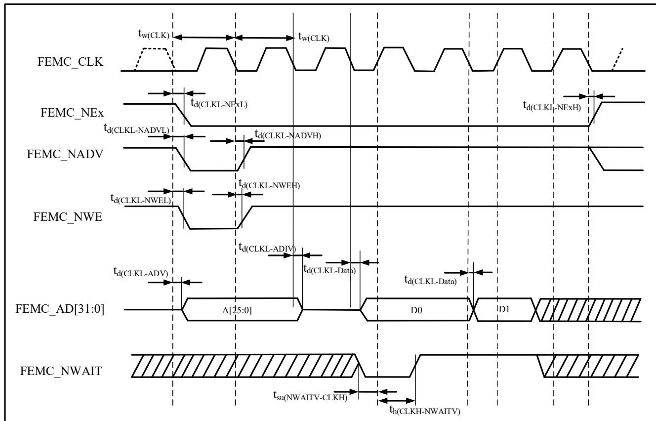
Table 4-59 Synchronous Multiplexed PSRAM Write Timing<sup>(1)(2)</sup>
