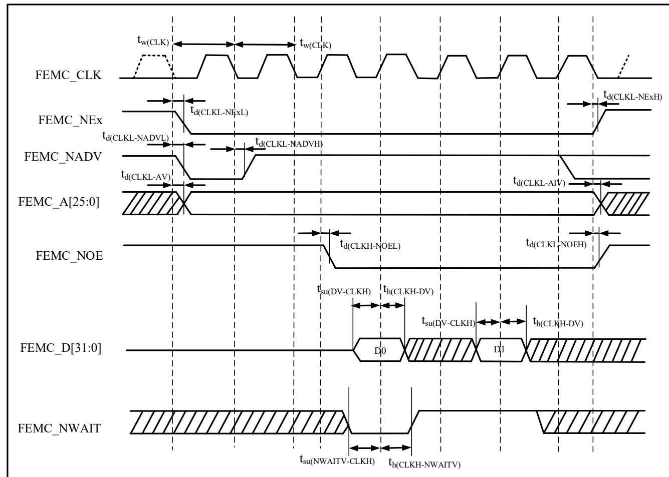
Table 4-56 Synchronous Non-Bus-Multiplexed NOR/PSRAM Read Timing<sup>(1)(2)</sup>
