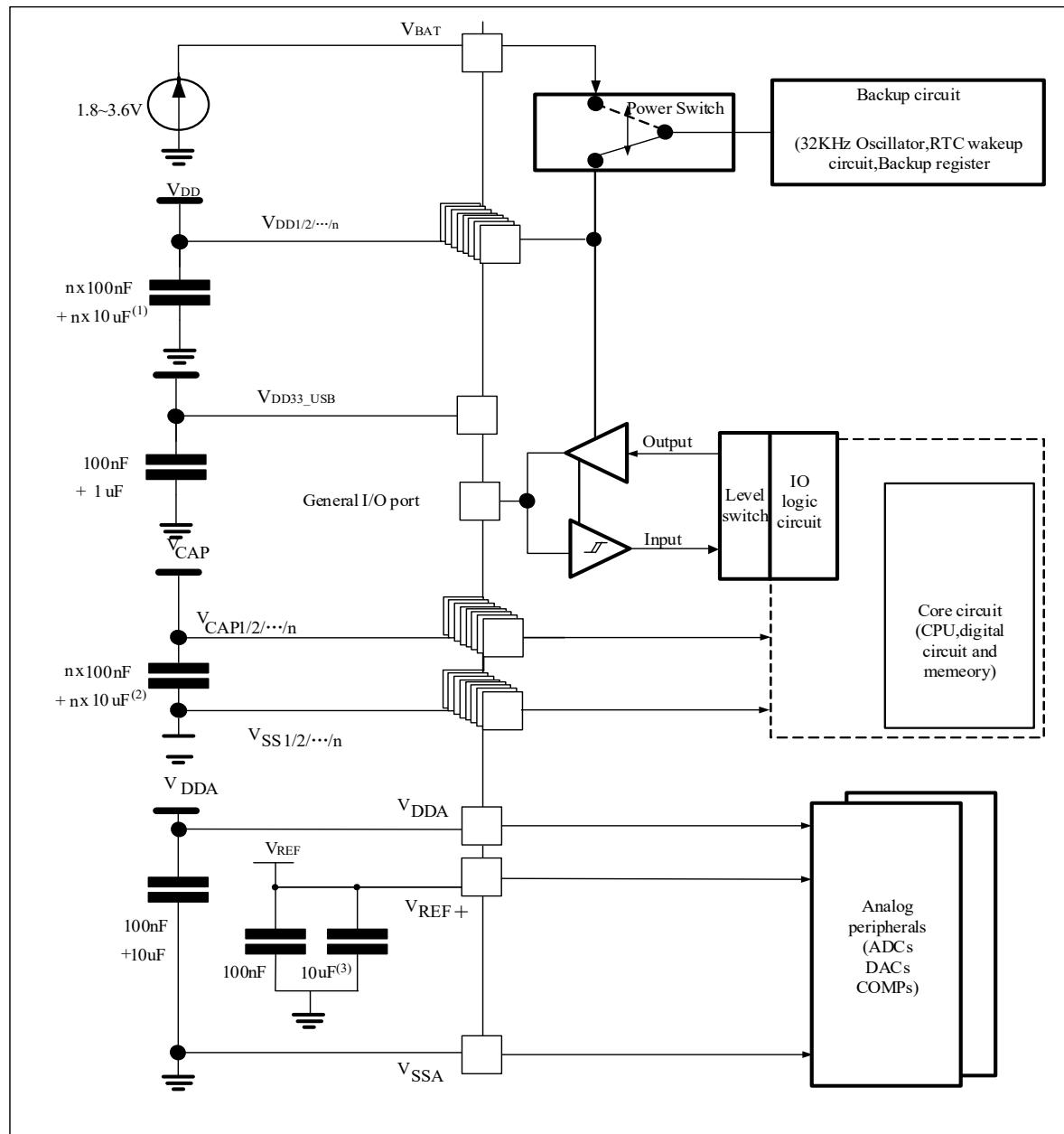
Note: 1. The  $10\mu F$  capacitor in the above figure must be connected to the specified VDD.
