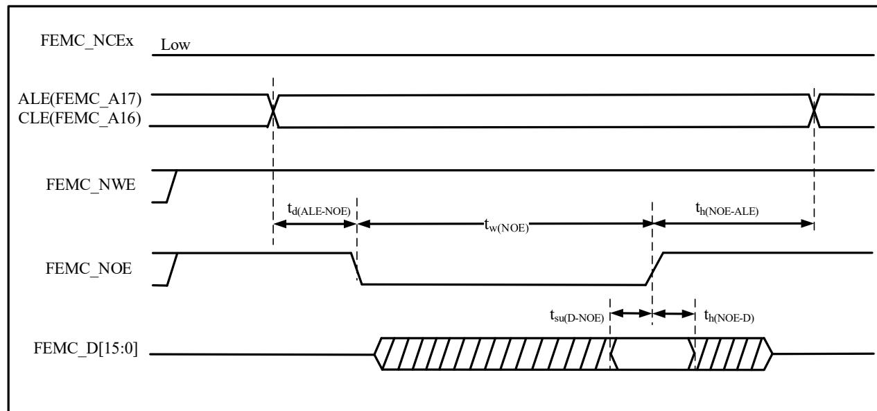
Figure 4-38 NAND Controller Write Operation Waveform
