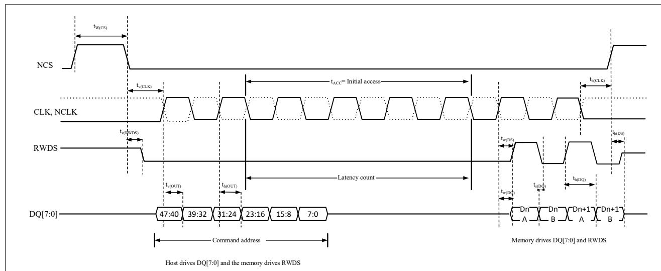
Figure 4-26 xSPI Hyperbus Clock Write Timing Diagram
