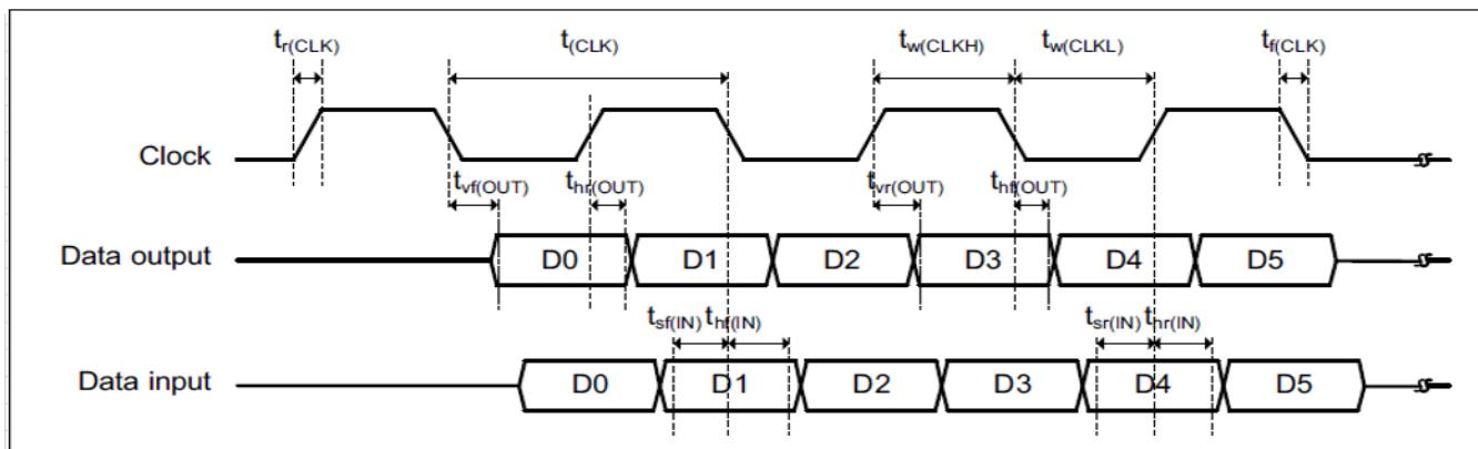
Table 4-51 xSPI Characteristics in DTR Mode (with DQS)/Eight-line and Hyperbus Protocol<sup>(1)</sup>
