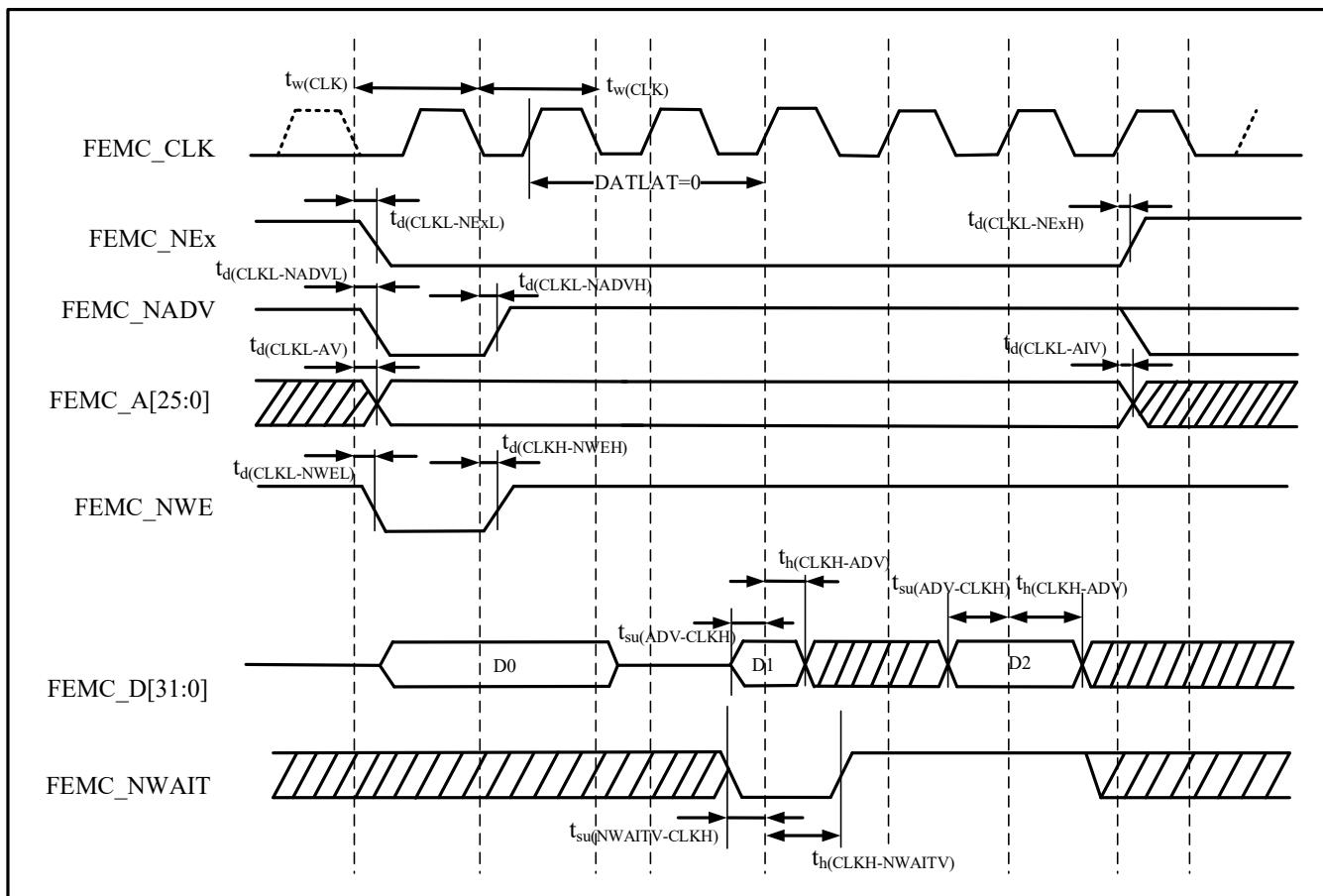
Table 4-57 Synchronous Non-Multiplexed PSRAM Write Timing (1)(2)
