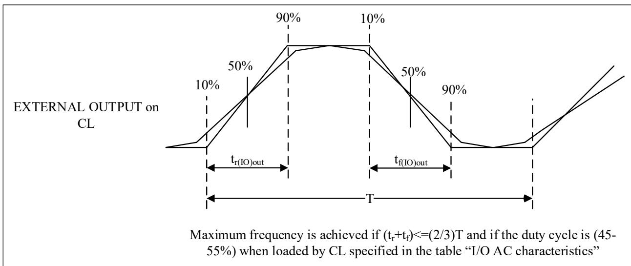
Figure 4-12 Transmission Delay
