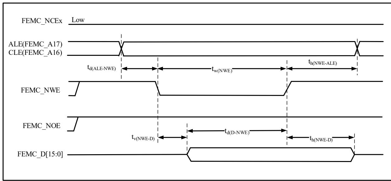
Table 4-60 NAND Flash Read Cycle Timing Characteristics<sup>(1)</sup>
