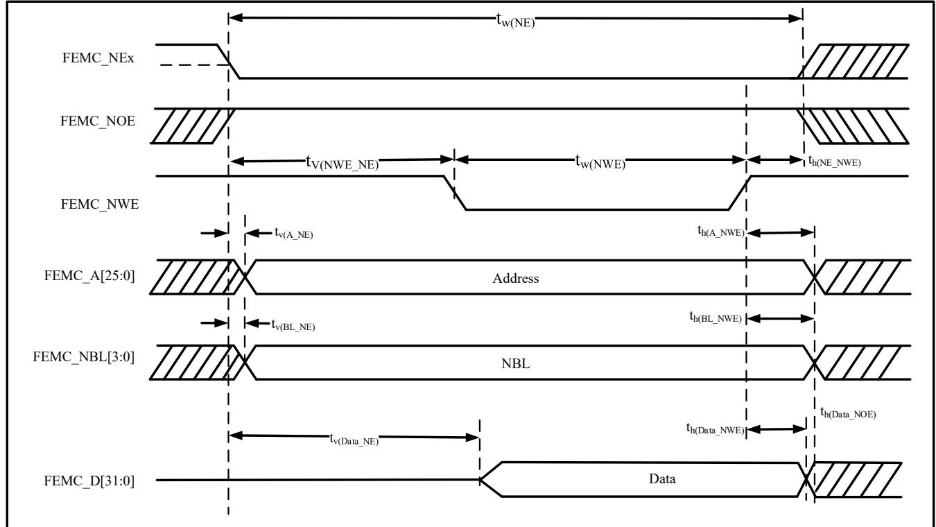
Table 4-53 Asynchronous Non-Multiplexed Bus SRAM/PSRAM/NOR Write Operation Timing<sup>(1)(2)</sup>
