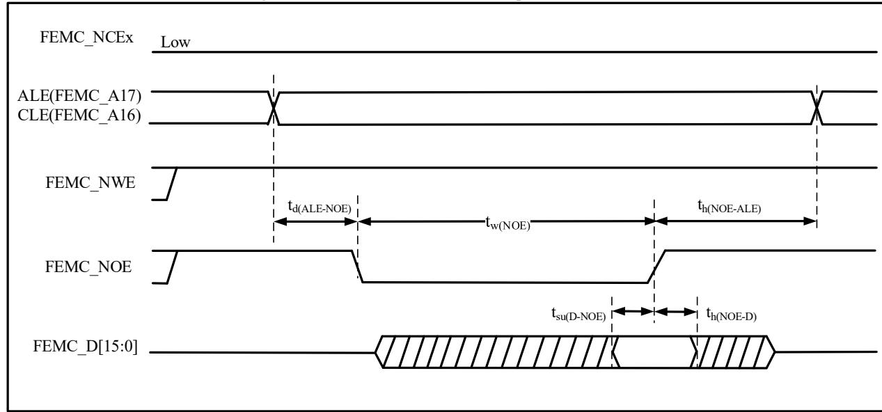
Figure 4-38 NAND Controller Write Operation Waveform
