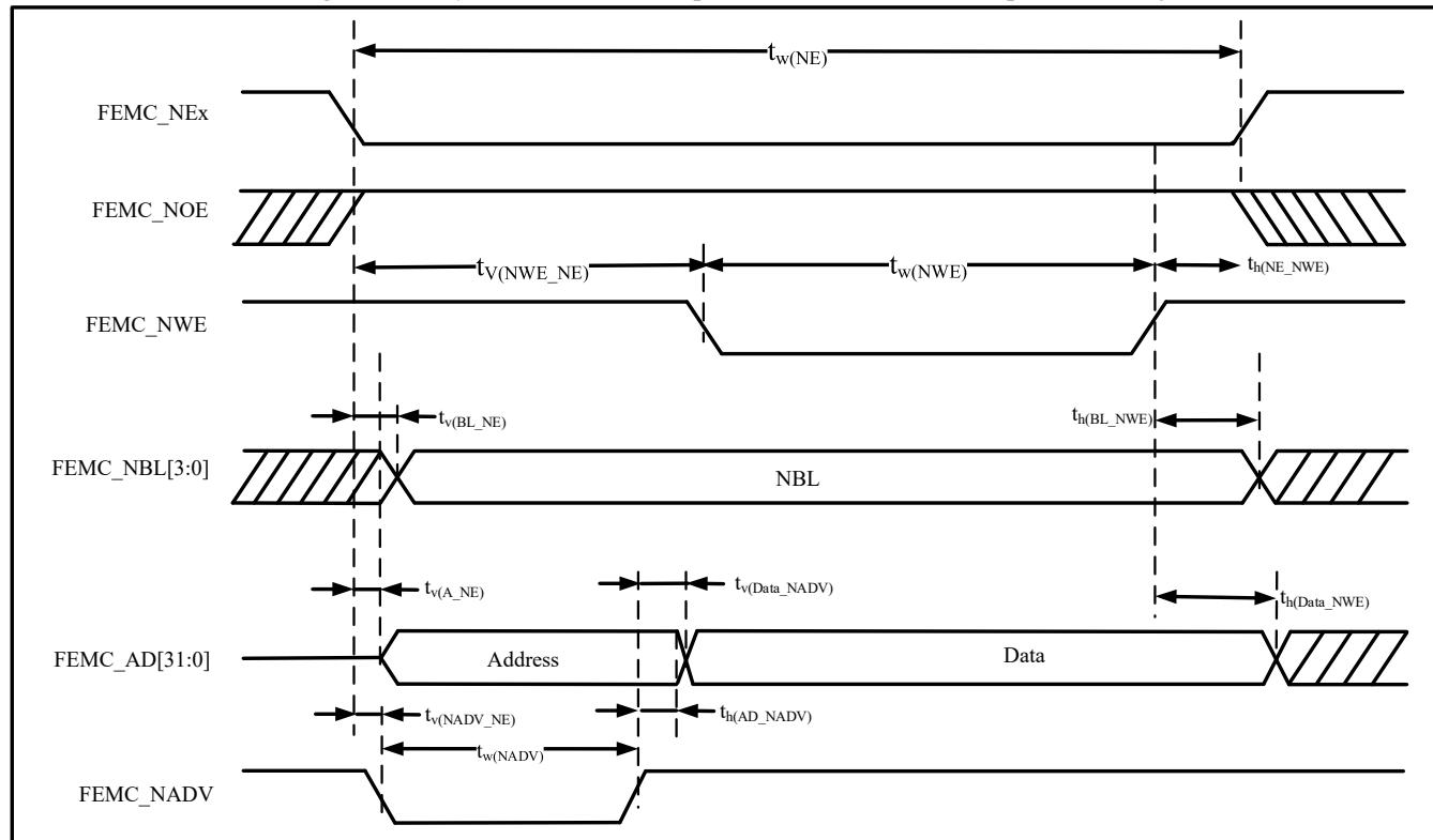
Table 4-55 Asynchronous Bus-Multiplexed PSRAM/NOR Read Operation Timing<sup>(1)(2)</sup>
