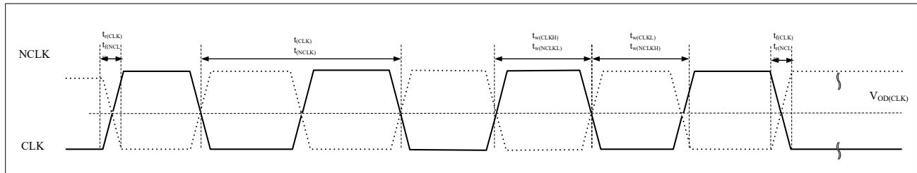
Figure 4-24 xSPI Hyperbus Clock Read Timing Diagram
