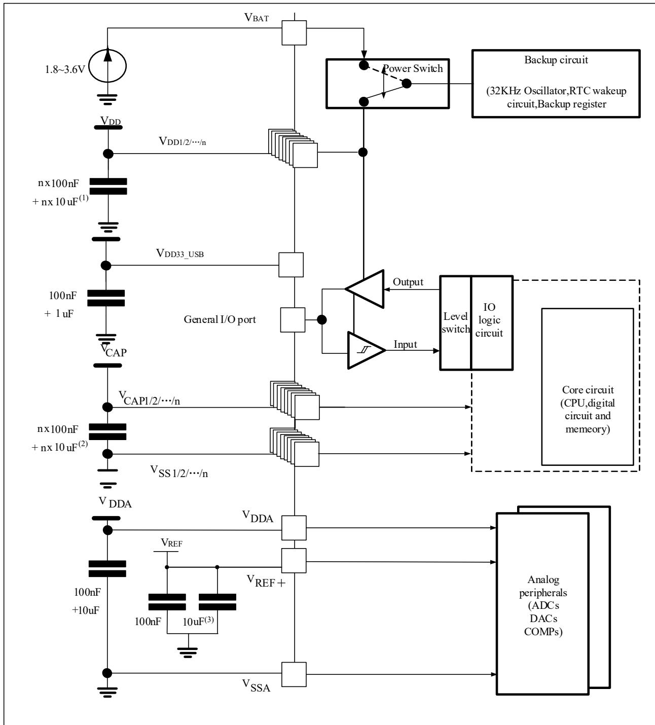
Note: 1. The 10μF capacitor in the above figure must be connected to the specified VDD.
