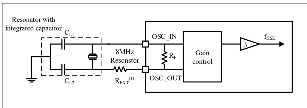
1. The value of  $R_{EXT}$  is determined by the characteristics of the crystal.
