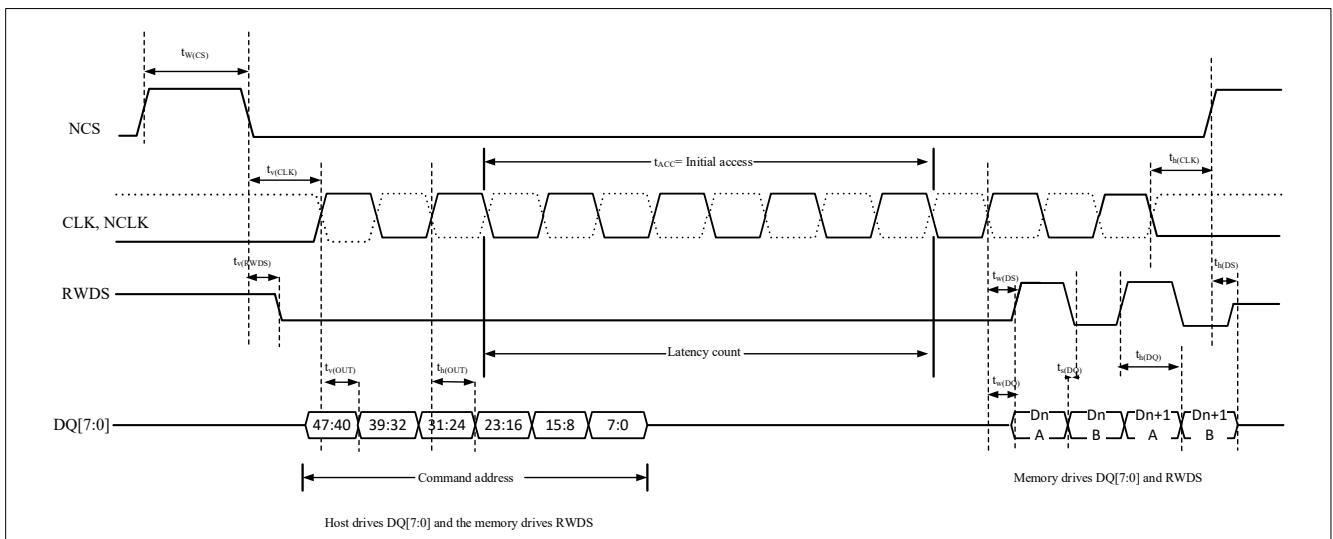
Figure 4-25 xSPI Hyperbus Clock Write Timing Diagram
