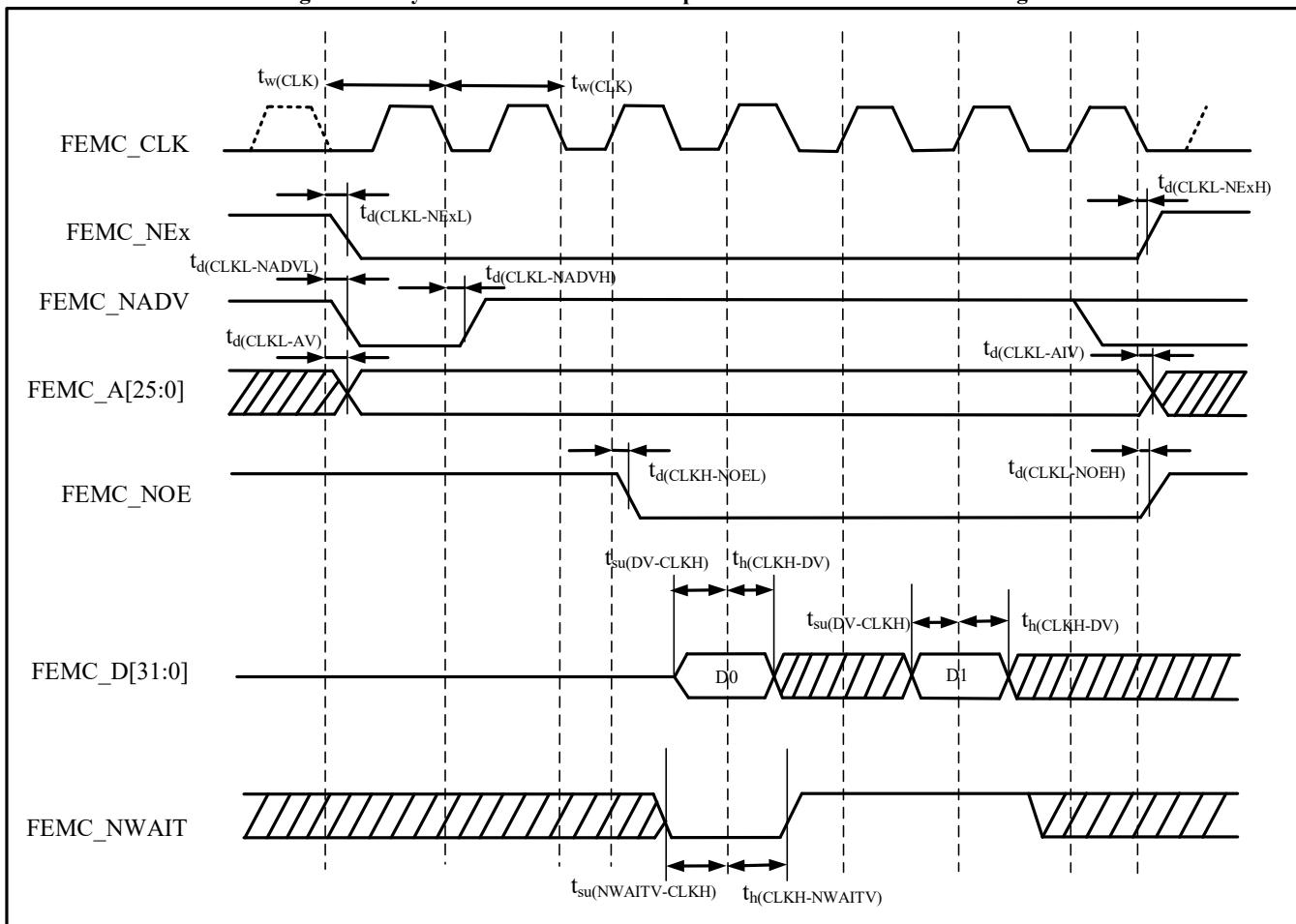
Table 4-56 Synchronous Non-Bus-Multiplexed NOR/PSRAM Read Timing<sup>(1)(2)</sup>
