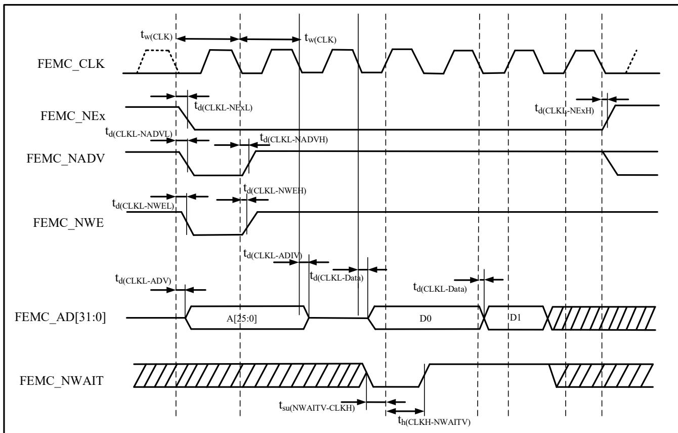
Table 4-59 Synchronous Multiplexed PSRAM Write Timing<sup>(1)(2)</sup>
