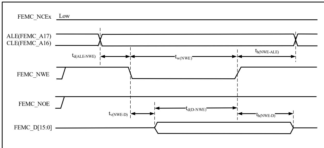
Table 4-62 NAND Flash Read Cycle Timing Characteristics <sup>(1)</sup>
