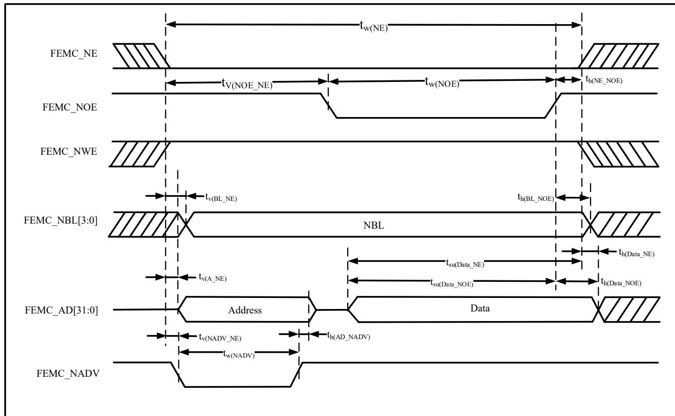
Table 4-54 Asynchronous Bus Multiplexed PSRAM/NOR Read Timing<sup>(1)(2)</sup>
