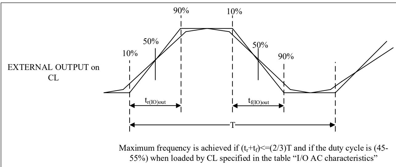
Figure 4-2 Transmission Delay
