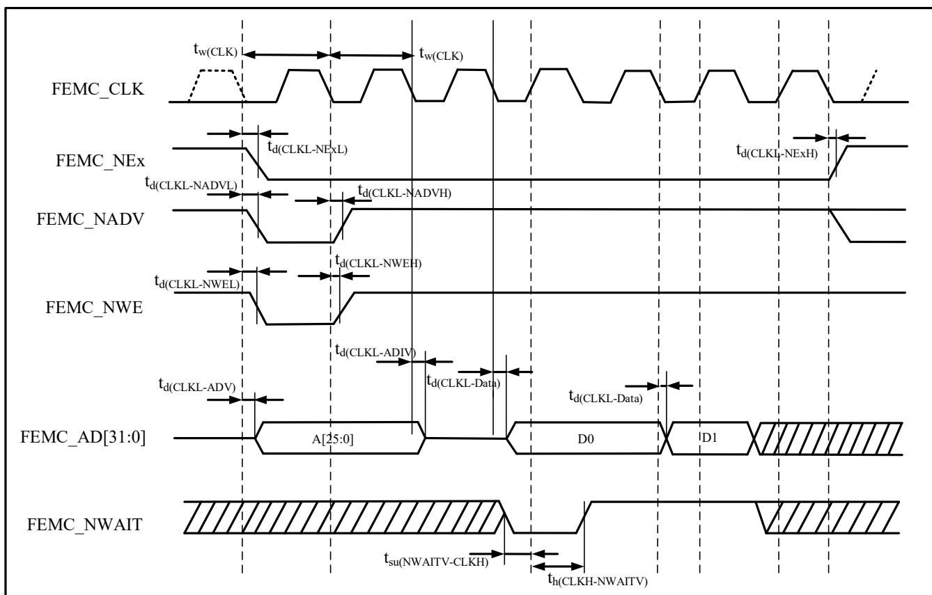
Table 4-52 Synchronous Multiplexed PSRAM Write Timing<sup>(1)(2)</sup>
