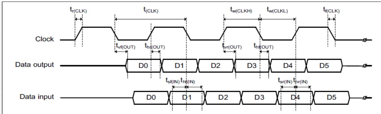
Table 4-44 xSPI Characteristics in DTR Mode (with DQS)/Eight-line and Hyperbus Protocol<sup>(1)</sup>
