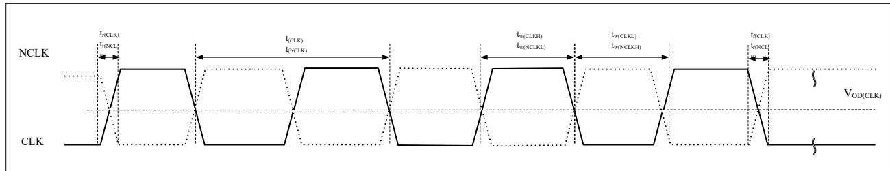
Figure 4-24 xSPI Hyperbus Clock Read Timing Diagram4-5 xSPI Hyperbus
