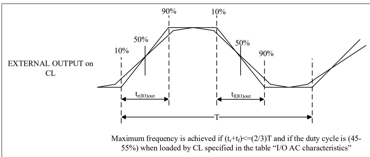
Figure 4-3 Transmission Delay
