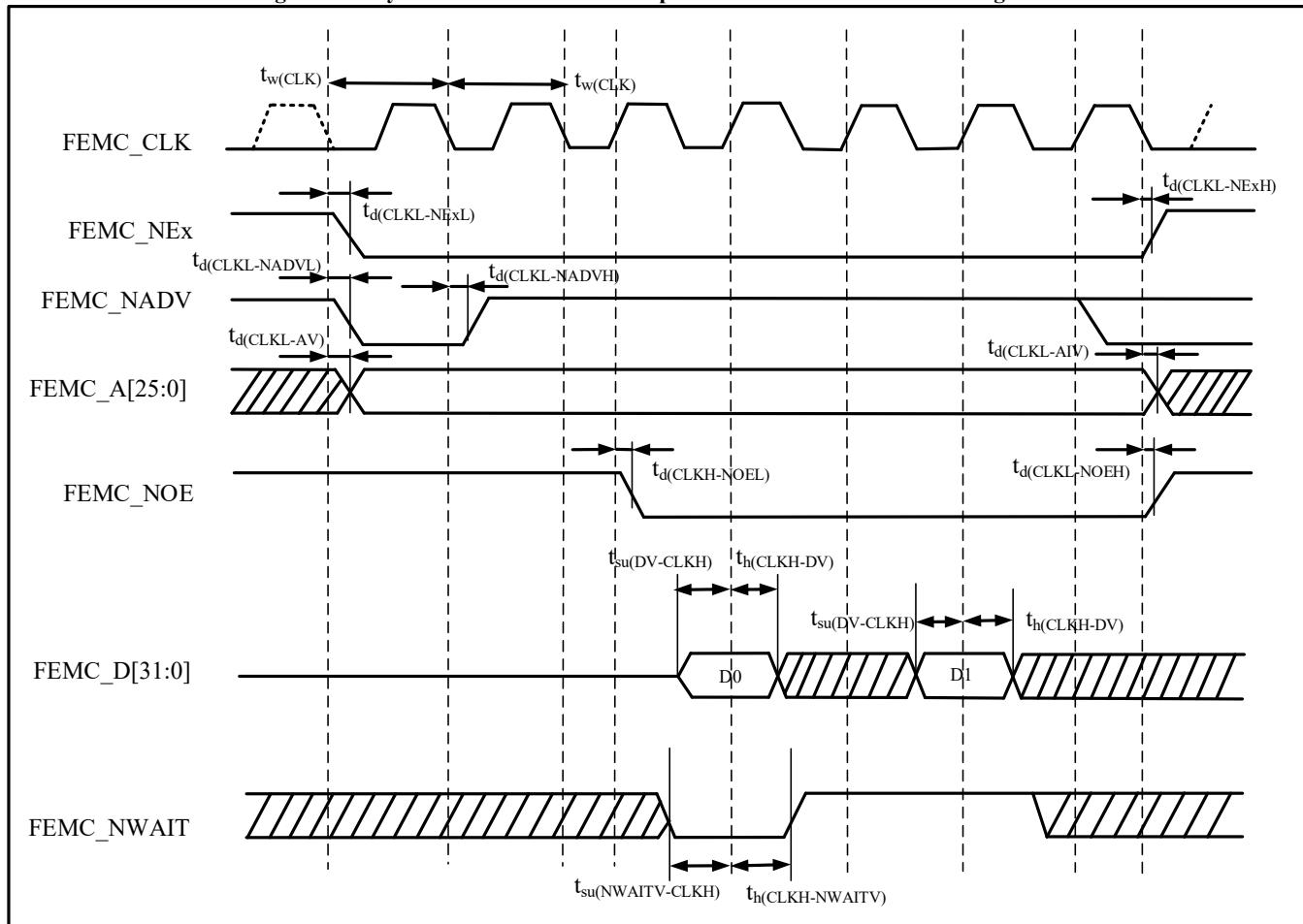
**Table 4-49 Synchronous Non-Bus-Multiplexed NOR/PSRAM Read Timing<sup>(1)(2)</sup>**
