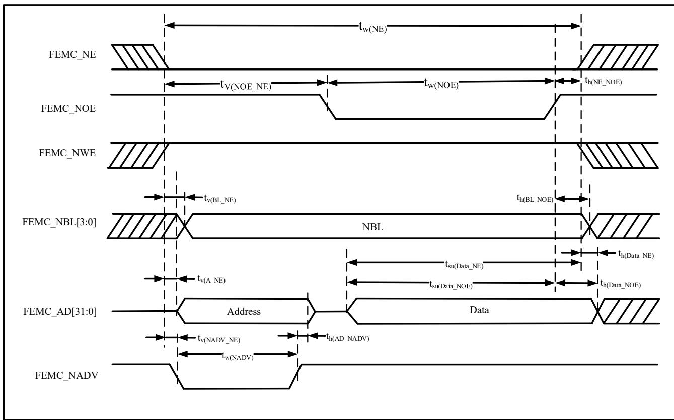
Table 4-7 Asynchronous Bus-Multiplexed PSRAM/NOR Read Operation Timing<sup>(1)(2)</sup>
