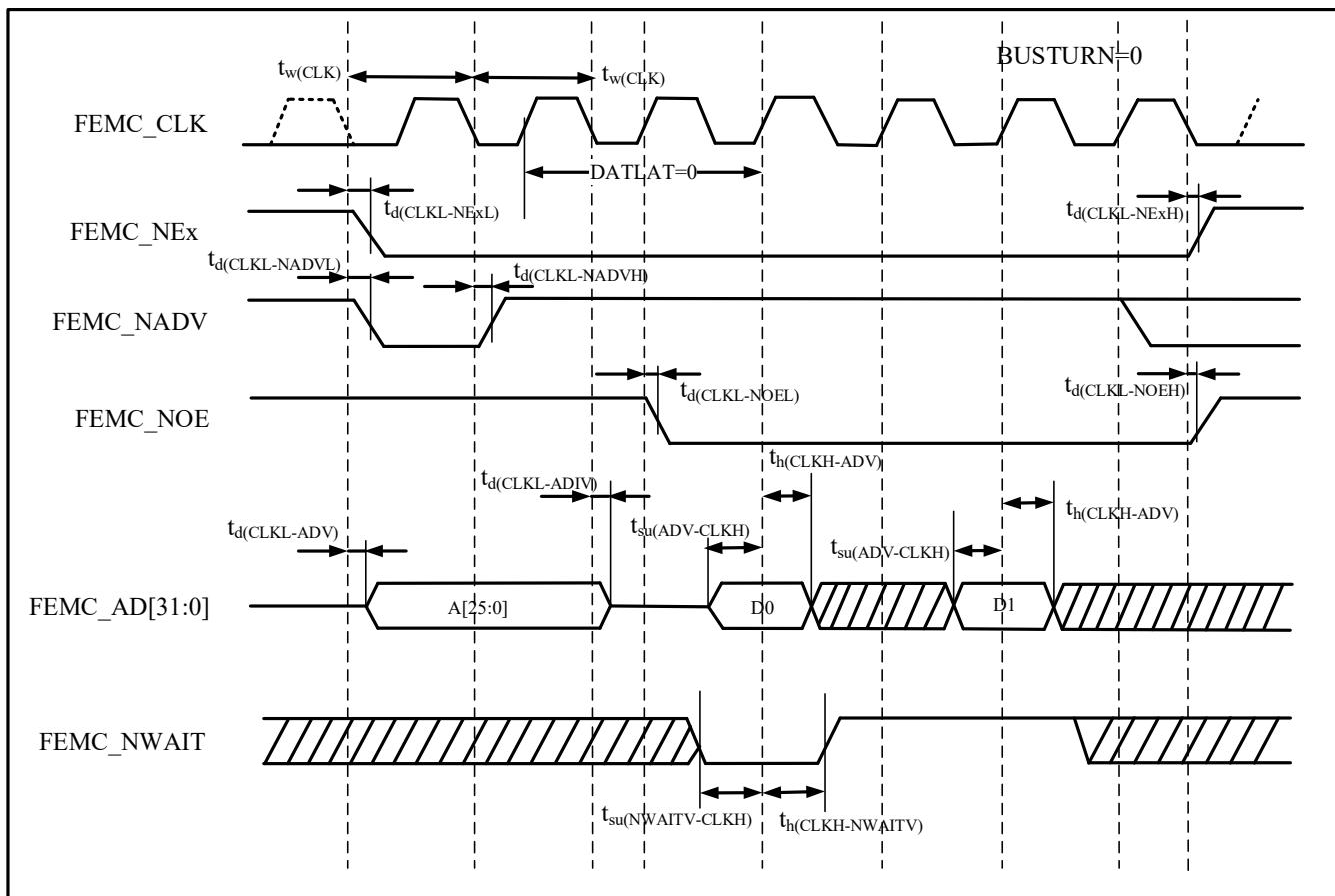
Table 4-51 Synchronous Bus-Multiplexed NOR/PSRAM Read Timing<sup>(1)(2)</sup>
