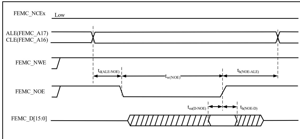
Figure 4-39 NAND Controller Write Operation Waveform
