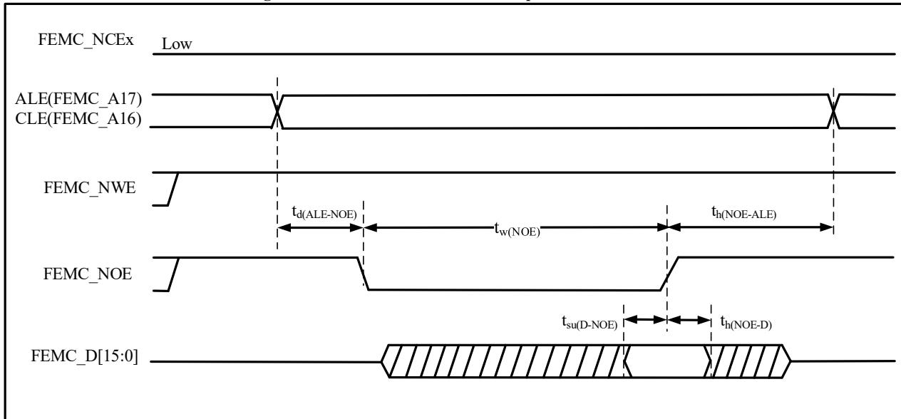
Figure 4-37 NAND Controller Write Operation Waveform
