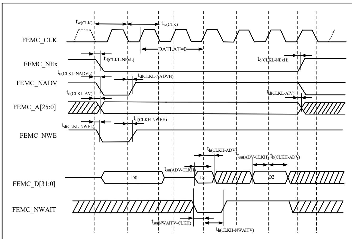
Table 4-50 Synchronous Non-Multiplexed PSRAM Write Timing<sup>(1)(2)</sup>
