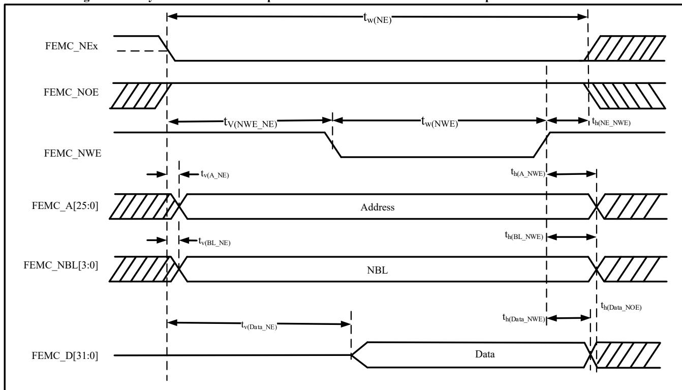
Table 4-46 Asynchronous Non-Multiplexed Bus SRAM/PSRAM/NOR Write Operation Timing<sup>(1)(2)</sup>
