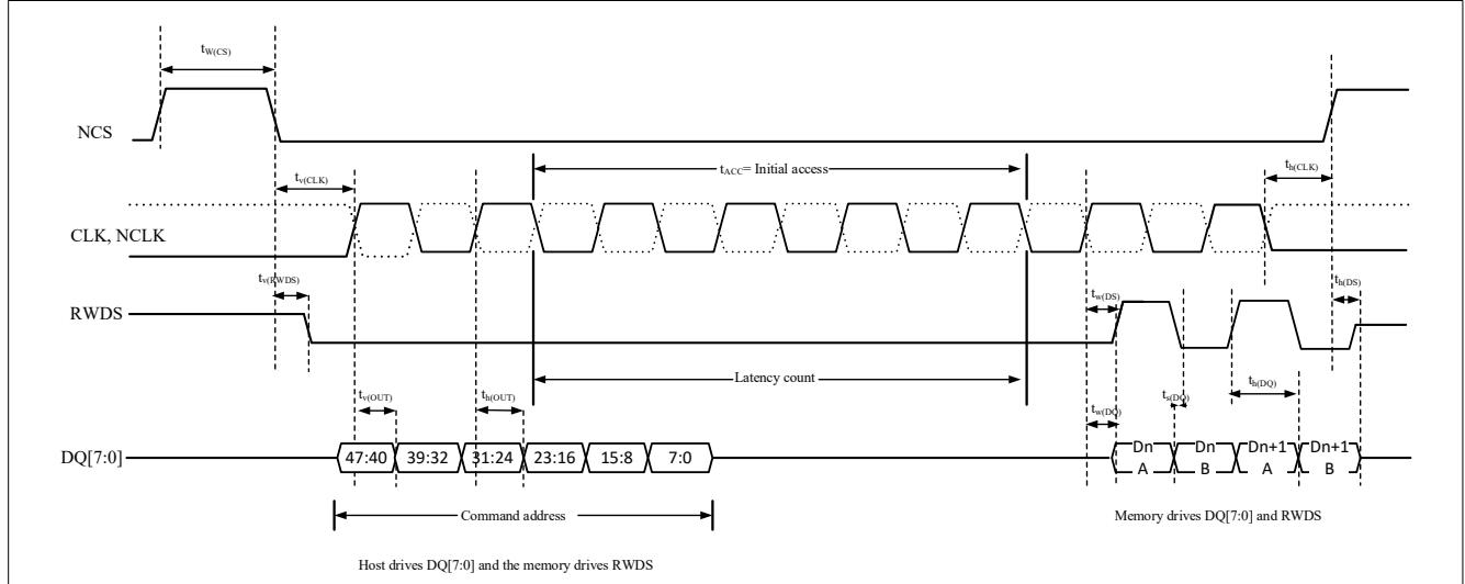
Figure 4-25 xSPI Hyperbus Clock Write Timing Diagram4-6 xSPI Hyperbus
