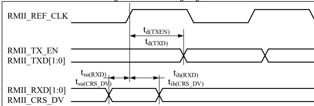
Table 4-63 lists the Ethernet MAC timing of MII and Figure 4-45 shows the corresponding timing diagram.
