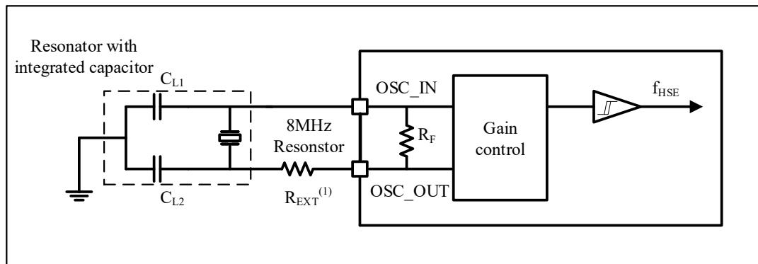
1. The value of R<sub>EXT</sub> is determined by the characteristics of the crystal.
