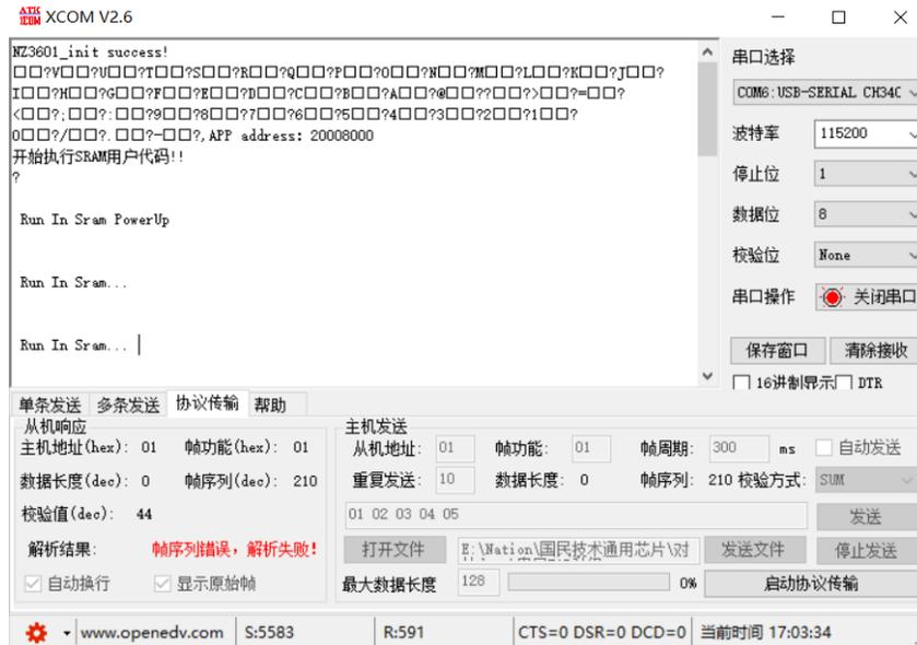
As shown in Figure 3-4, after receiving the BIN file, the program successfully jumped to APP\_address: 0x20008000 to execute the code in Sram.
