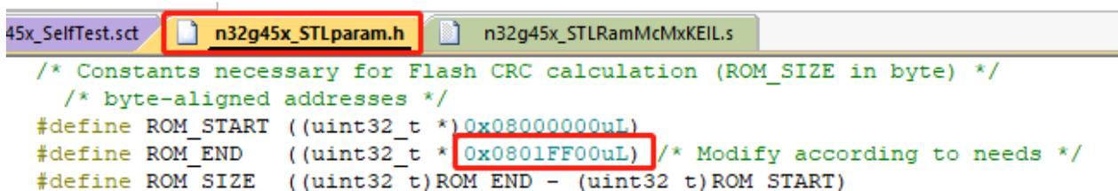
Therefore, whether it is downloading or debugging, the final generated N32G45x\_SelfTest\_CRC.hex file needs to be used, so the .ini file needs to be added to the Keil configuration option to download the new .hex file. The configuration is as follows:
