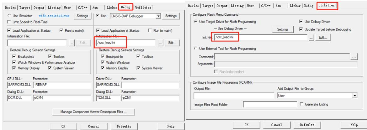
It should be noted that the .ini file should also modify the content file name configuration according to the actual application:
