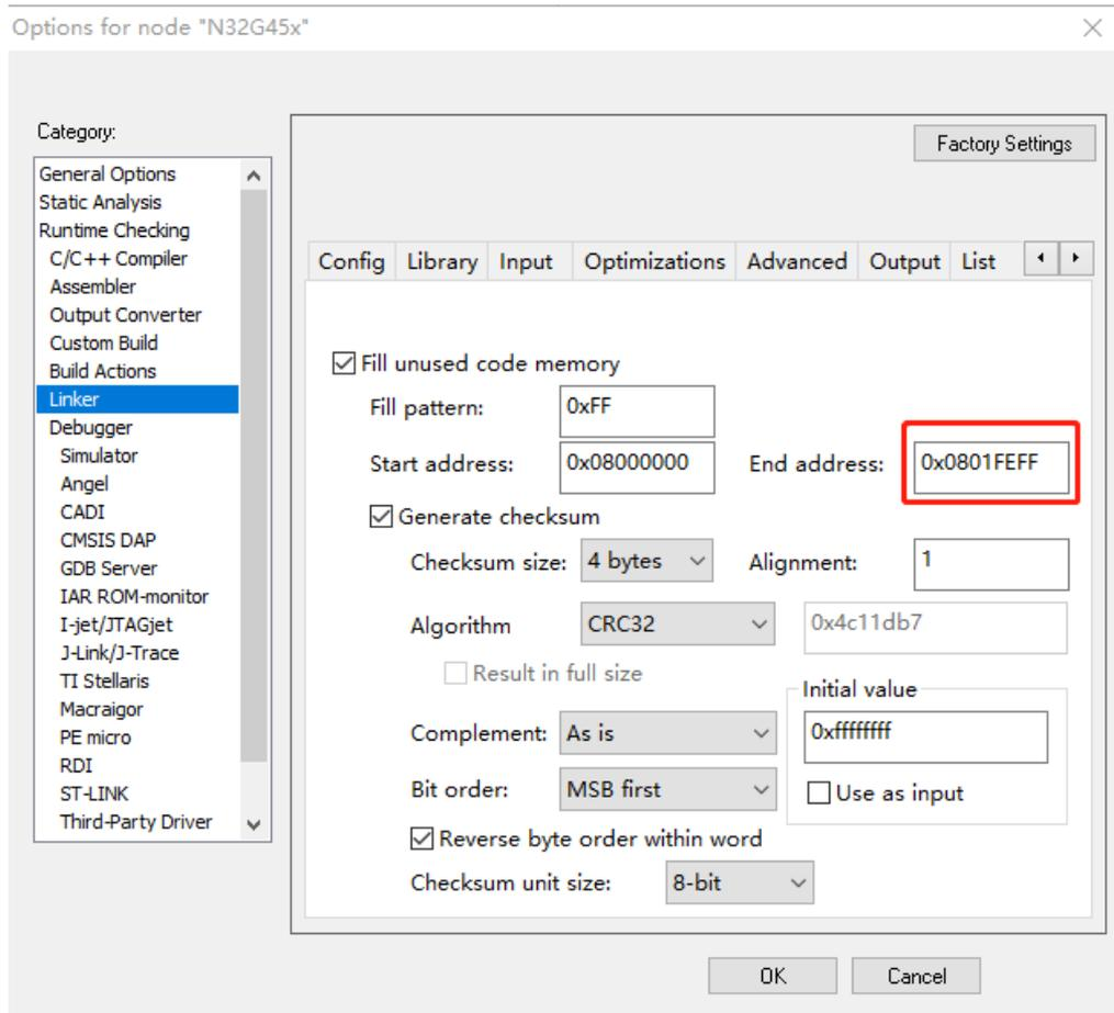
The range of calculating CRC in the program is configured according to the .icf file, which can be modified according to the needs. Add 4 to the above configuration:
