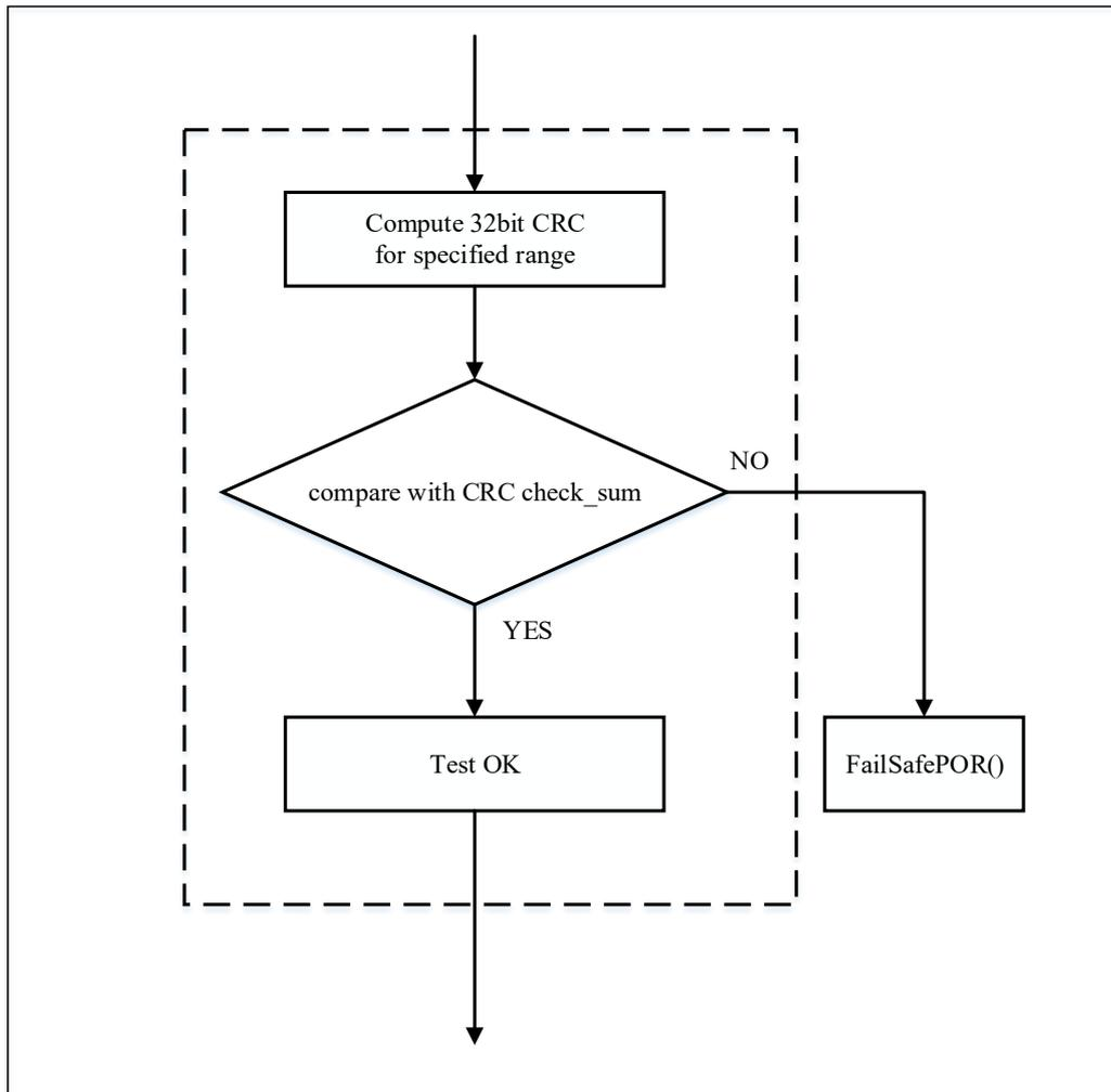
FLASH range of CRC calculation is configured according to the actual situation of the whole program, and the method is different on KEIL and IAR.
